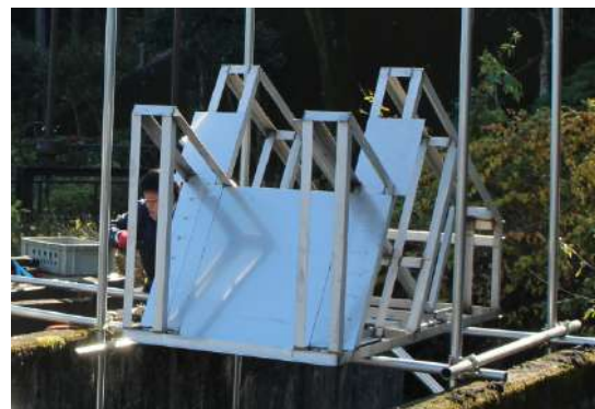
The steel plate (Block Plate) blocks the flow of water to level up the water surface to the hydraulic head.
