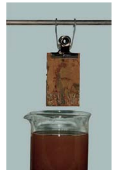
Rock wool Many Corrosion of about 600µm depth can be seen.
